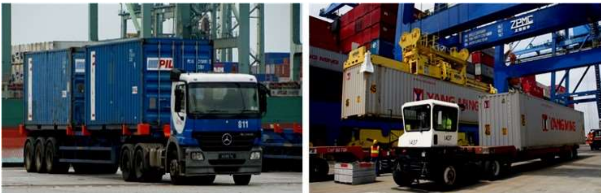
Figure 7.13 Typical ITV for Handling Containers
