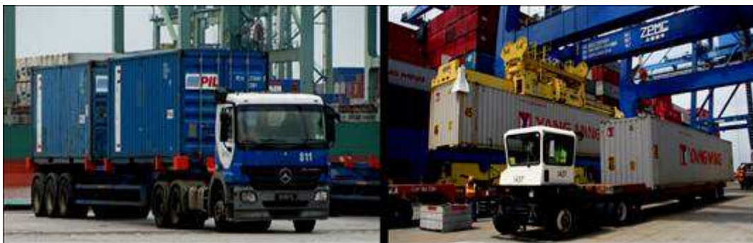
Figure 7.9 Typical ITV for Handling Containers
