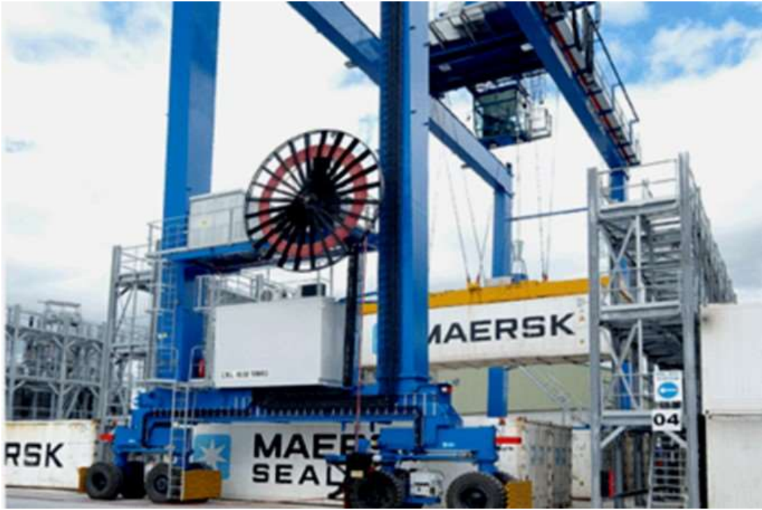
Figure 7.9 Typical E-RTG for Yard Operation
