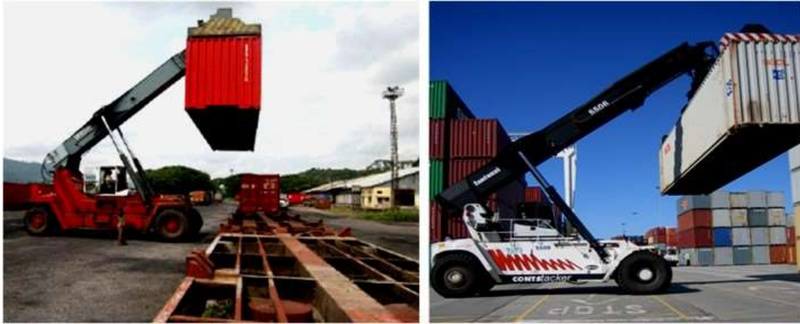
Figure 7.12 Snapshot of Typical Reach Stacker Handling
