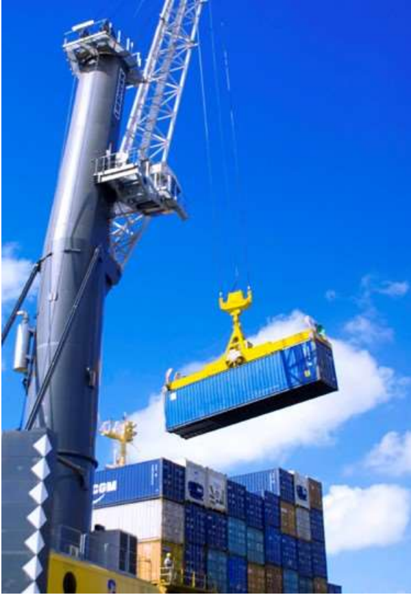
Figure 7.8 Mobile Harbour Crane with Spreader Arrangement
