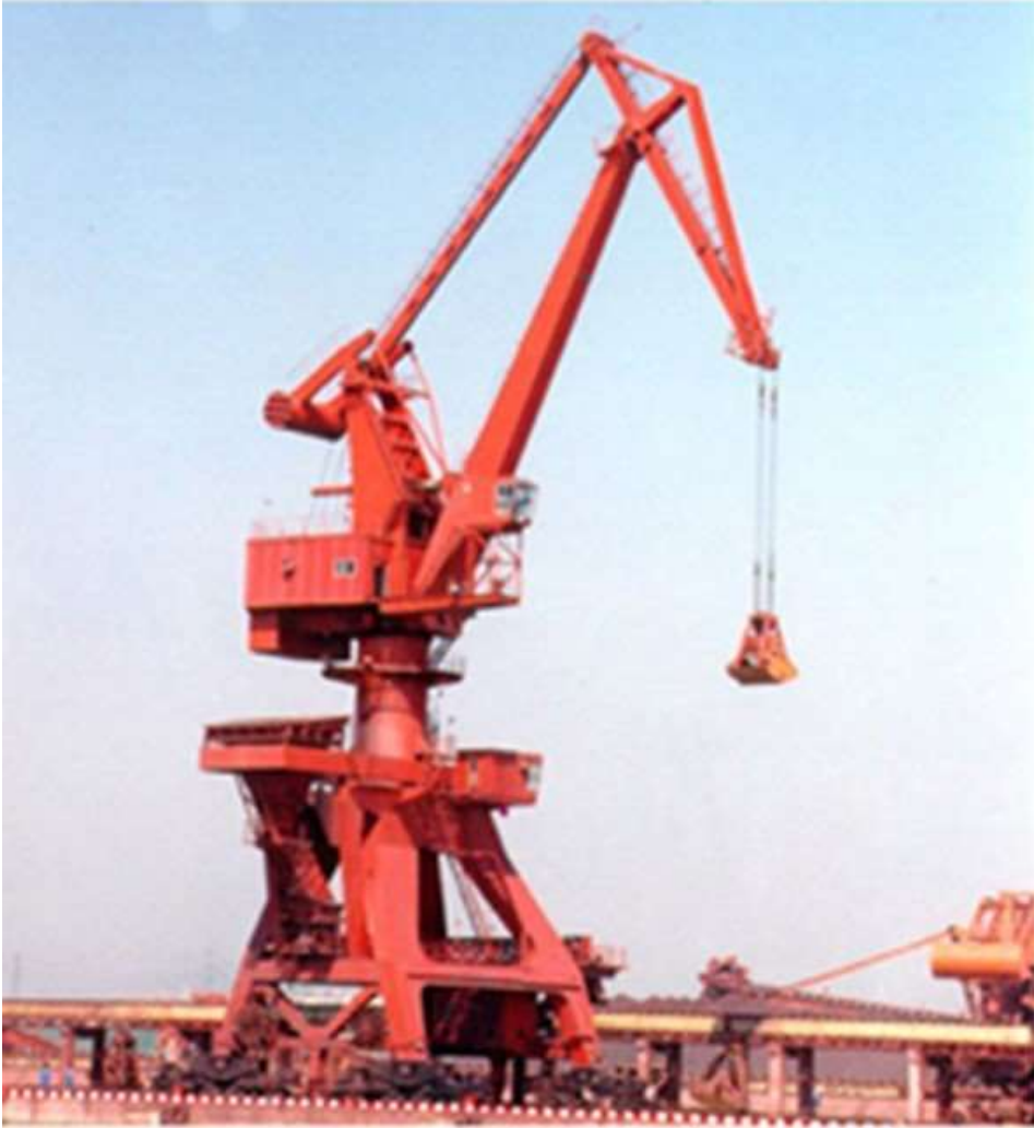
Figure 4.1 Typical Arrangement of Mobile Harbour / ELL Cranes with Mobile Hopper
