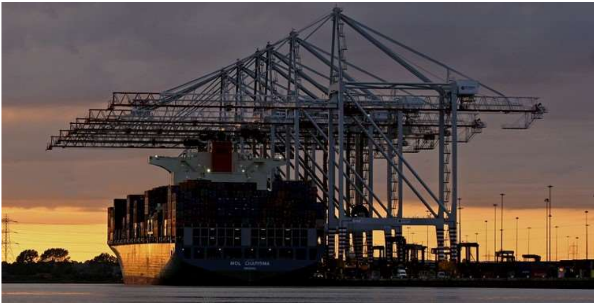
Figure 7.9 Typical RMQCs Operating at Berth
