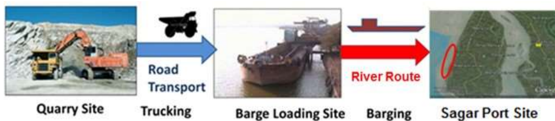
Figure 7.7 Logistics Flow diagram from Quarry to Port Site
