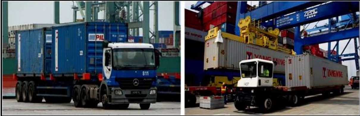
Figure 7.15 Typical ITV for Handling Containers
