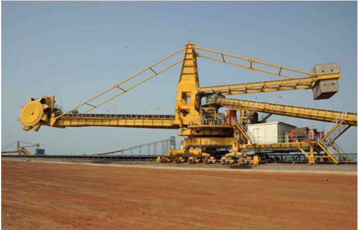
Figure 7.24 Typical Stacker cum Reclaimer
