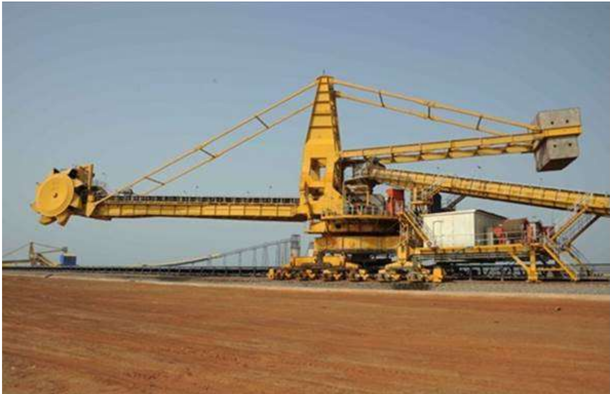
Figure 7.2 Typical Stacker cum Reclaimer
