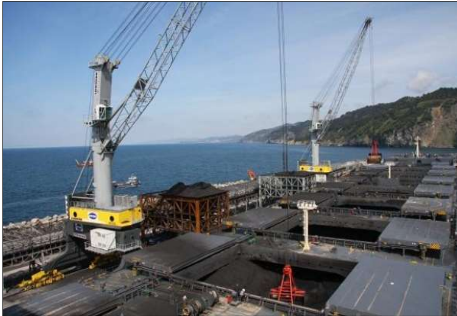
Figure 7.8 Typical Mobile Harbour Cranes with Mobile Hoppers
