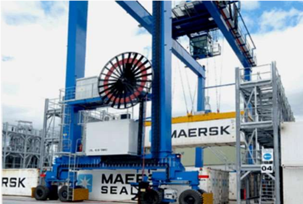
Figure 7.10 Typical E-RTG for Yard Operation
