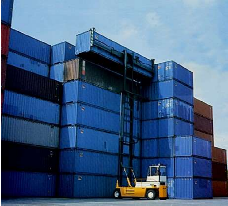
Figure 7.13 Snapshot of Typical Side-pick Handling
