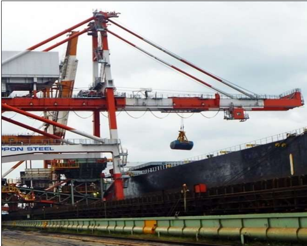
Figure 7.23 Typical Ship Unloader
