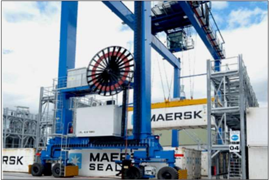
Figure 7.25 Typical E-RTG for Yard Operation
