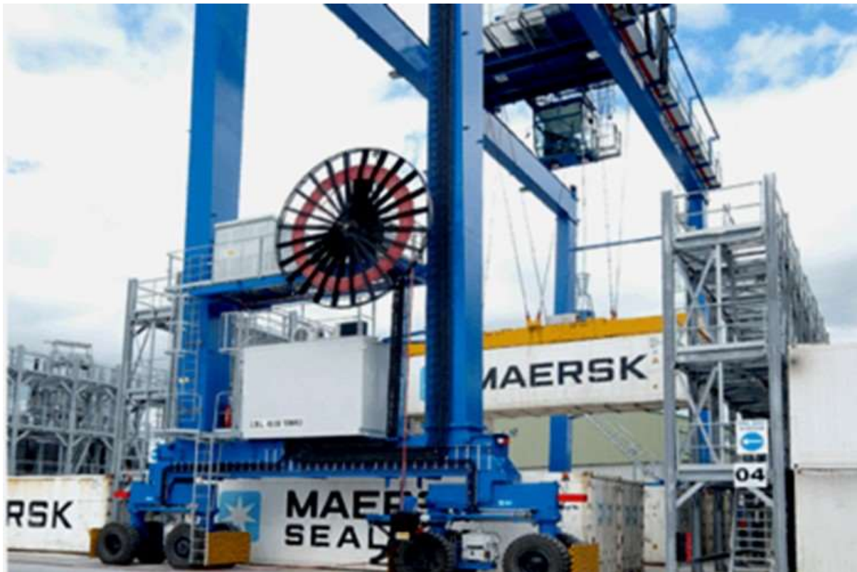
Figure 8.18 Typical E-RTG for Yard Operation
