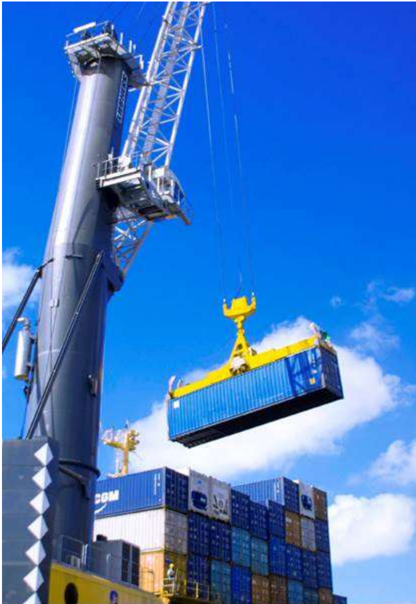
Figure 7.4 Mobile Harbour Crane with Spreader Arrangement
