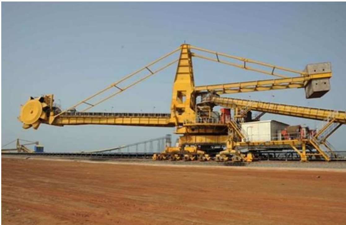
Figure 8.15 Typical Stacker cum Reclaimer
