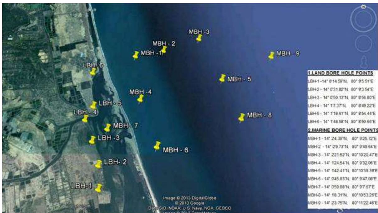
Figure 2.6 Location Plan of Land and Marine Boreholes
