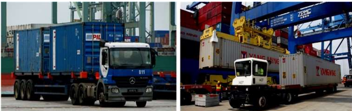
Figure 8.22 Typical ITV for Handling Containers
