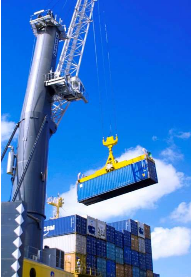
Figure 8.17 Mobile Harbour Crane with Spreader Arrangement
