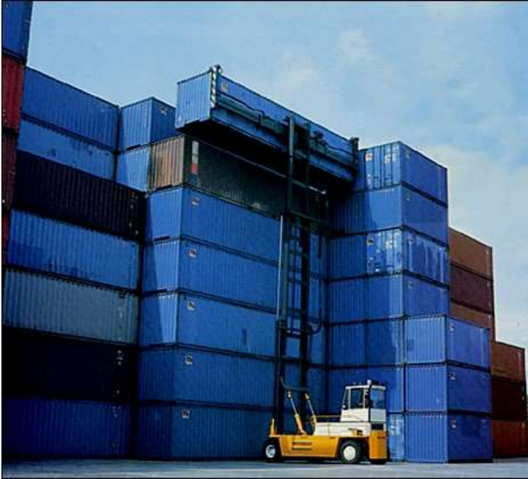
Figure 7.28 Snapshot of Typical Side-pick Handling Containers will be transported between the quay and the empty storage areas by ITVs.
