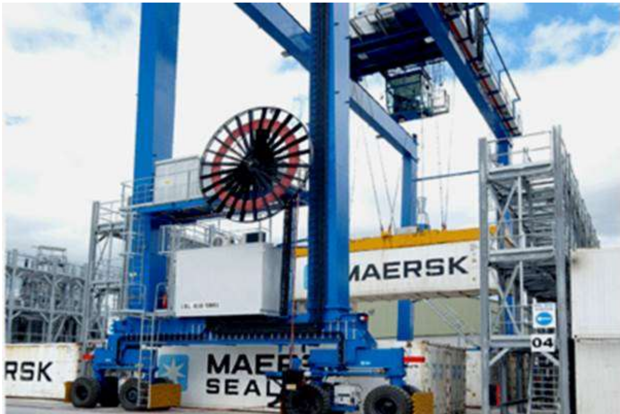
Figure 7.5 Typical E-RTG for Yard Operation
