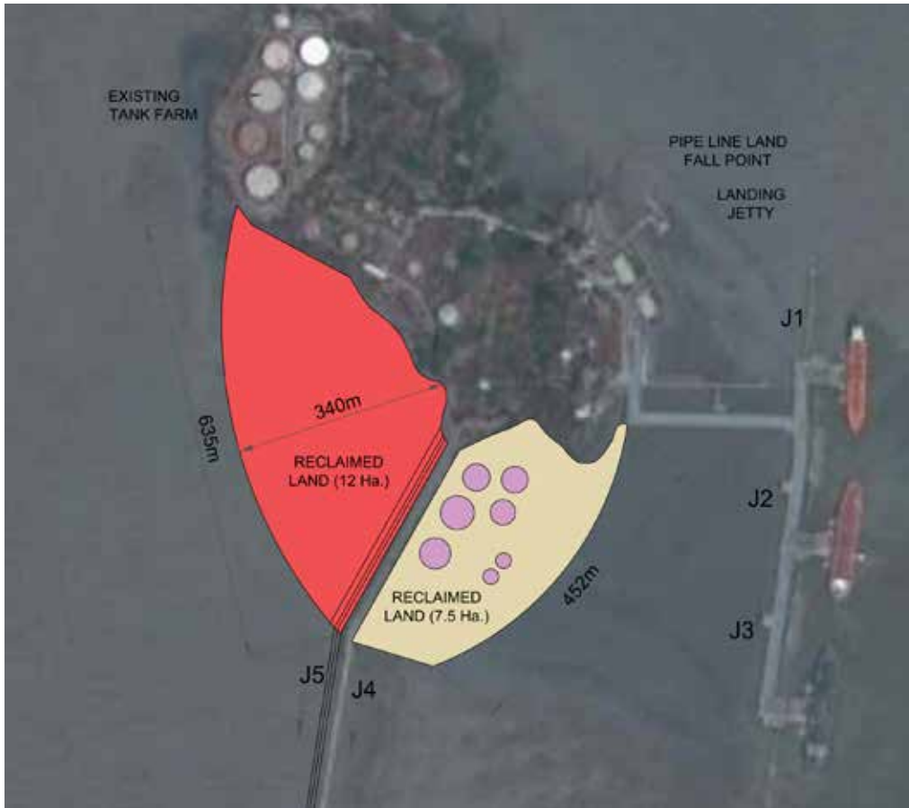
Figure 7.3 Proposed Reclamation for Additional Storage Tanks
