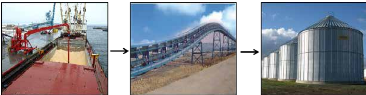
Figure 9.8 Mechanised Food Grain Unloading Facility
