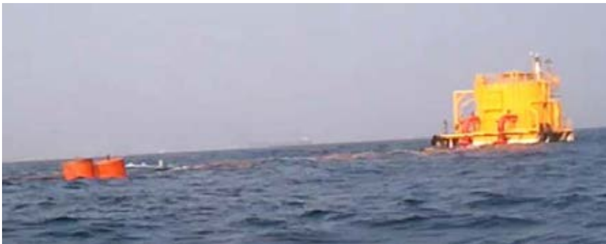
Figure 3.10 Turret Buoy with Floating Hoses
