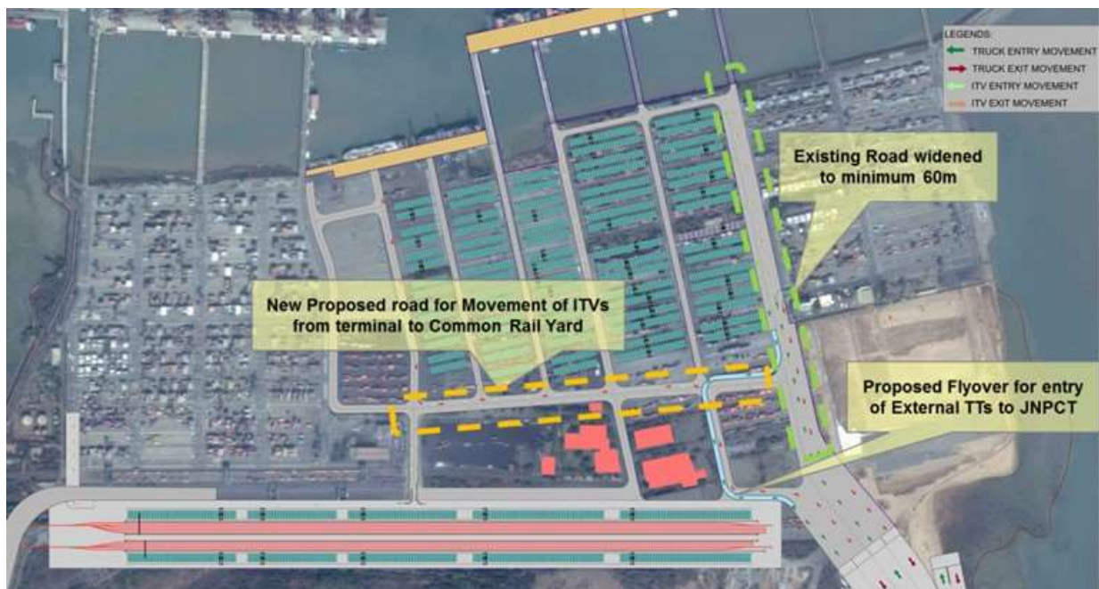
Figure 7.11 Major Changes in the Existing Layout for the Smooth Flow of Traffic at the Container Terminal
