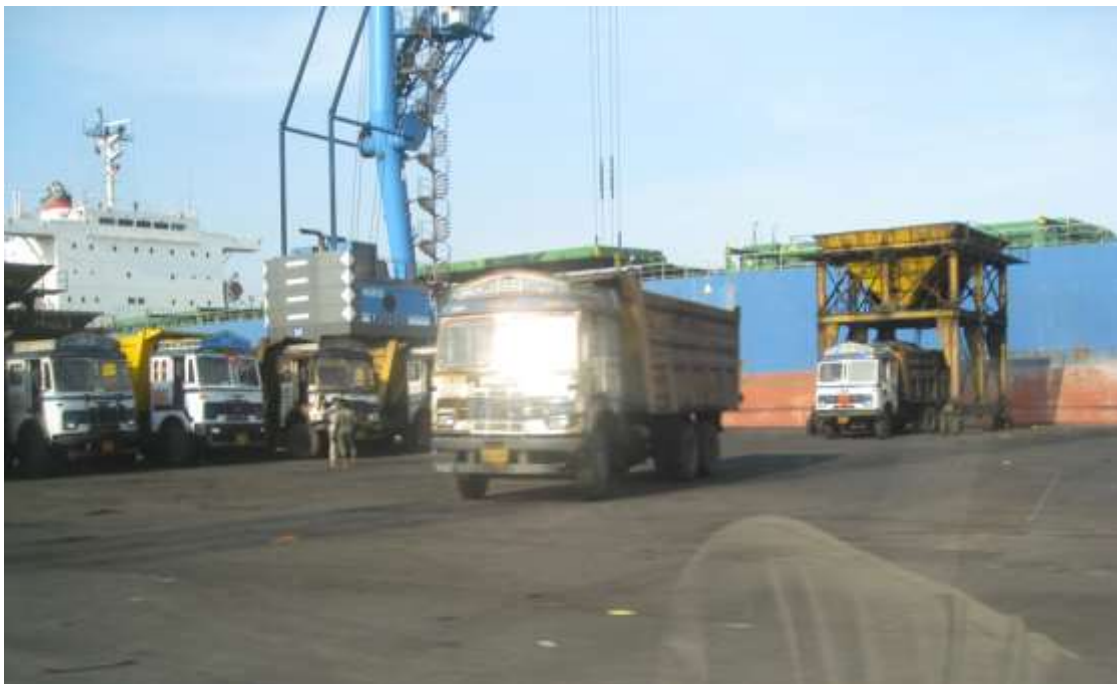
Figure 9.2 Loading of trucks through Hoppers
