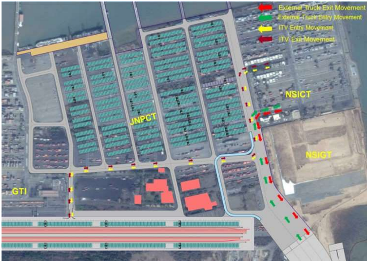
Figure 7.12 Traffic Circulation Plan for NSICT Terminal
