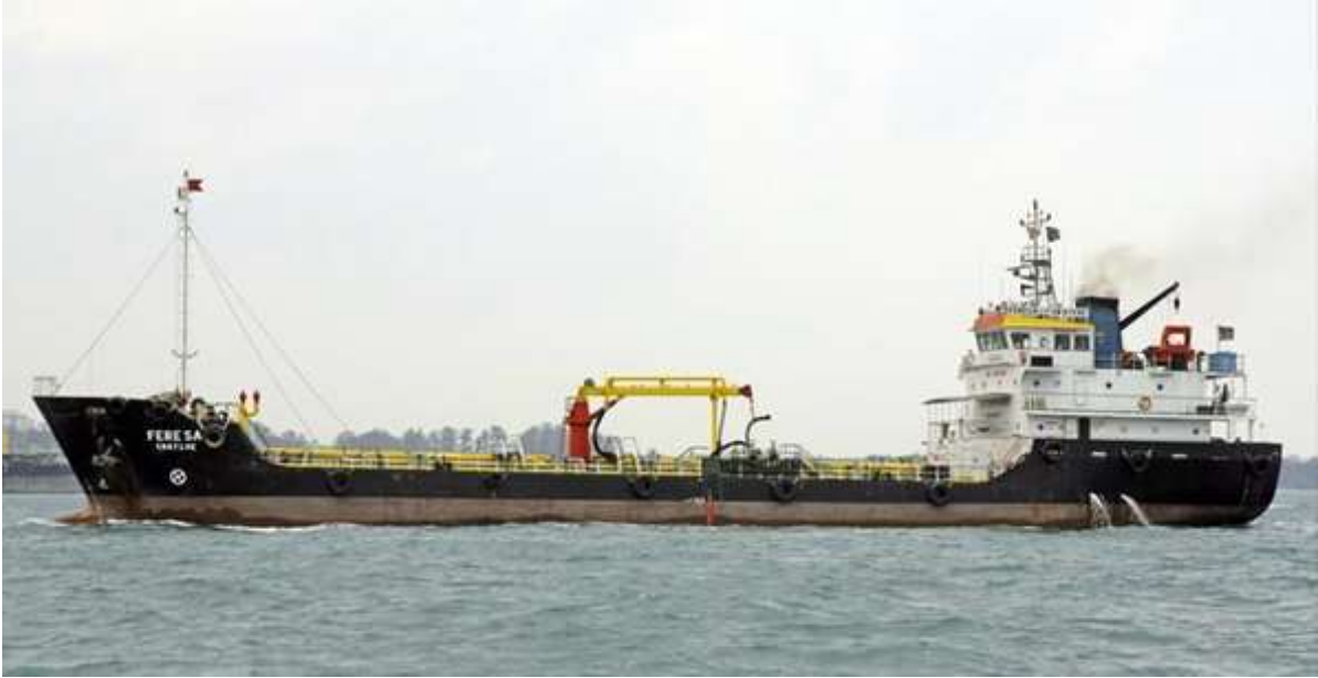
Figure 1.22 A Typical 1,600 T Bunker Tanker
