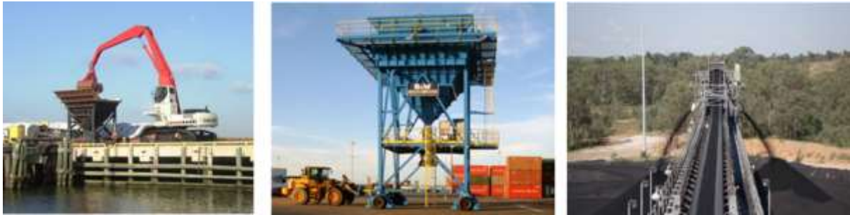
Figure 7.7 Typical Barge Unloading Equipment
