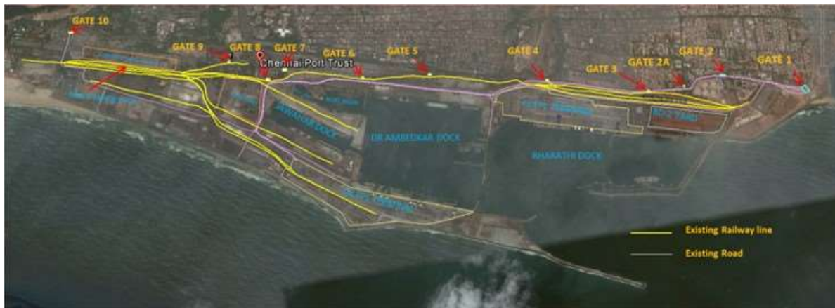
Figure 1.11 Overall Port Railway Network
