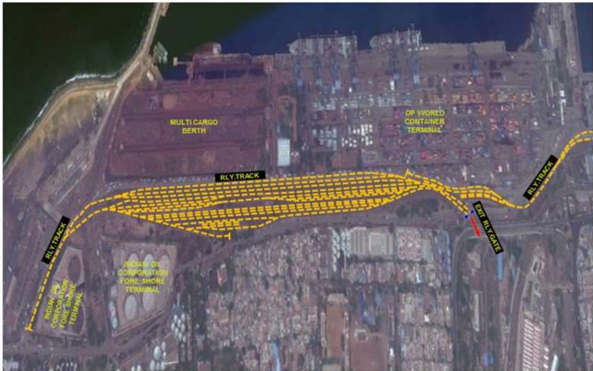
Figure 1.14 Railway Network at BD II Yard at Bharathi Dock
