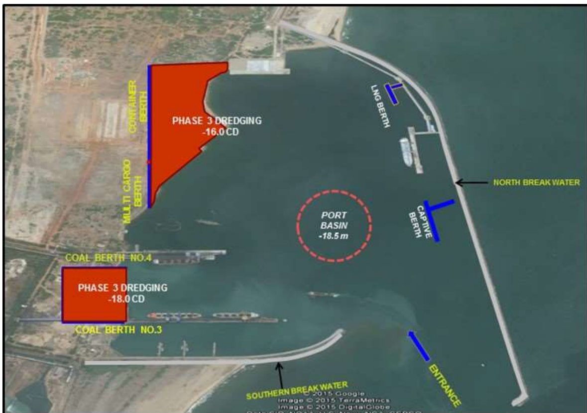
Figure 5.2 Phase 3 Capital Dredging
