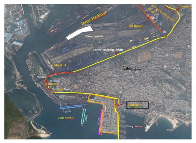
Figure 8.8 Outer Harbour Road with Critical Locations for Widening (4 Lane Road Proposal)
