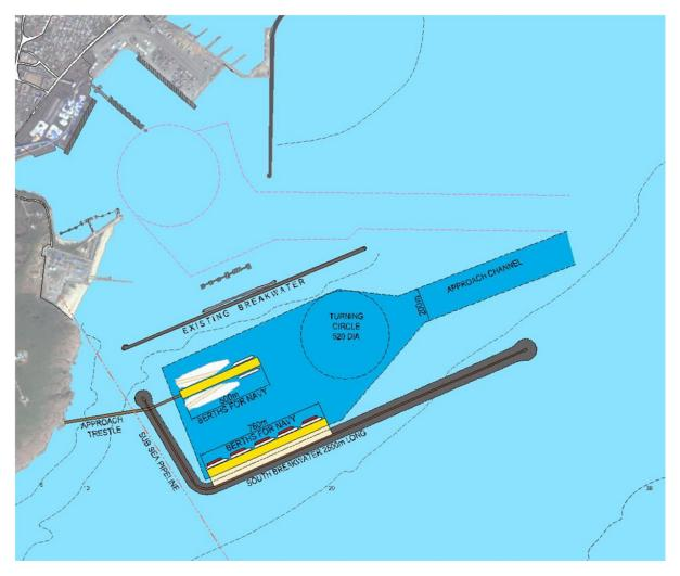
Figure 9.1 Proposed Outer Harbour - Layout Plan Alternative 1
