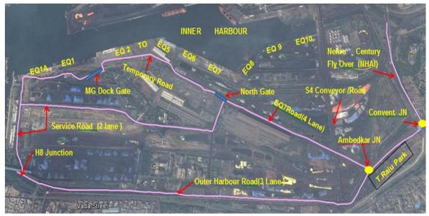
Figure 8.3 Connectivity of EQ 1A to EQ 7 Berths
