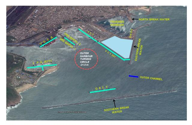
Figure 10.2 Layout of Outer Harbour alongwith Ongoing Developments
