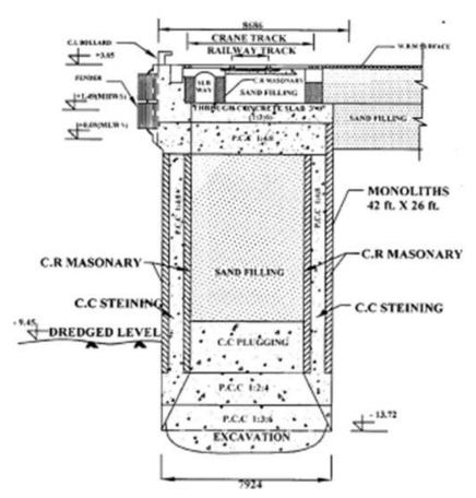
Figure 7.9 Cross Section of OR 1 & OR 2
