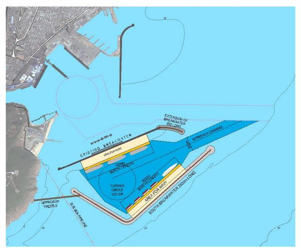
Figure 9.2 Proposed Outer Harbour - Layout Plan Alternative 2
