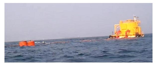
Figure 3.10 Turret Buoy with Floating Hoses
