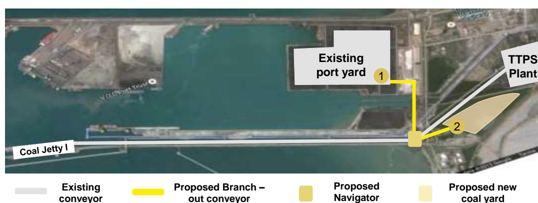
Figure 308: Layout for the proposed branch-out conveyor
