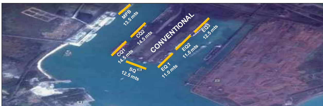
Figure 87: Conventional berths layout and draughts for respective berths at PPT
